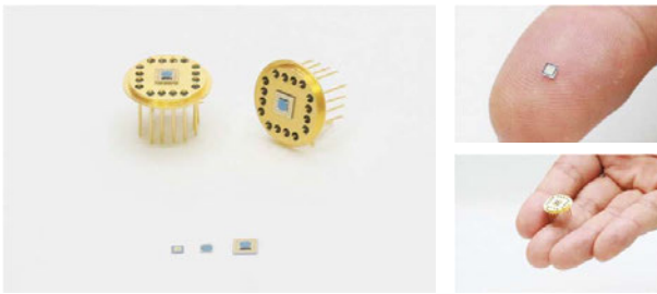
Fig. 6 Picture of the iPMSEL in TO-8 package.
