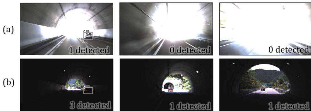
Fig. 9 Examples of object detection by each control method. (a) Conventional method A, (b) proposed method.
